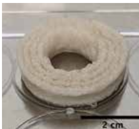
Whole scaffold of a fiber-based additive manufactured silk used to mimic an intervertebral disc. © Courtesy of Benjamin Gantenbein
